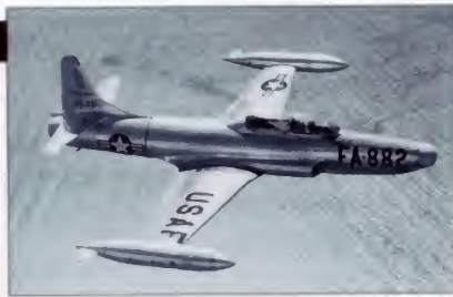
The earlier-production F-94B bore a stronger resemblance to the TF-80C (later redesignated T-33) from which it was developed. The F-94C introduced a swept tailplane, a broader rear fuselage and wing-mounted rocket pods.
